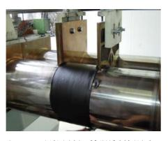
Step5: 測量並記錄膠料的溫度,最好低於 60 °C。 Measure and record the compound's temperature. Better below 60 °C.
