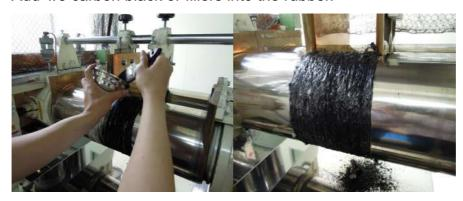
Step2: 持續清掃下方盤面,再將剩餘的碳黑加到滾動中原膠。 Clean the plate and put the rest of carbon black into the rubber.
