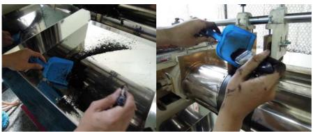
Step3: 混合均匀後,切下左側膠料一次,拉出部分膠料,再放入滾筒中。 Cut the left side of the compound, draw out a part of it, and put it back onto the rolls.
